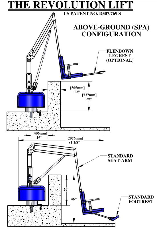
WITH THE SEAT MOUNTED AT ITS HIGHEST POSITION THE REVOLUTION LIFT WILL CLEAR A 29" [737mm] HIGH BY 12" [305mm] THICK WALL. THE SETBACK DISTANCE FOR THIS SITUATION IS 16" [406mm]. FOR OTHER APPLICATIONS AN OPTIONAL SPA SEAT-ARM IS AVAILABLE, MAKING IT POSSIBLE FOR THE REVOLUTION LIFT TO CLEAR UP TO A 48" [1219mm] HIGH WALL. AN OPTIONAL FLIP-DOWN LEGREST IS ALSO AVAILABLE FOR ABOVE-GROUND APPLICATIONS (SHOWN).
