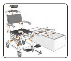
Ensure the primary brake securely locks your Tubbuddy + Tilt in position on the wheeled base before disconnecting the bridge.
