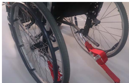
Fitting the Rear Restraint
