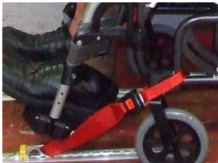
Fitting the front restraint
