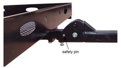
Insert the spring pull pin into the hole on the ramp when you stand the ramp. See the figure.
