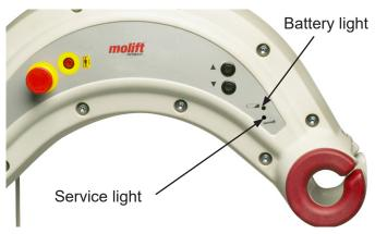
The electronics measures the operating time of the lifter, and after a specific time the yellow light will illuminate, indicating that the lifter needs service. Take contact with your local Molift service representative/dealer. The lifter can still be operated, but after a while an audible alarm will sound, to remind the operator that the lifter needs service immediately.
