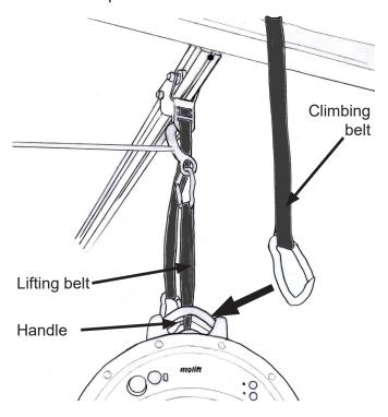
• Raise the lifter until it is possible to attach the climbing belt on the opposite trolley to the lifters handle.
