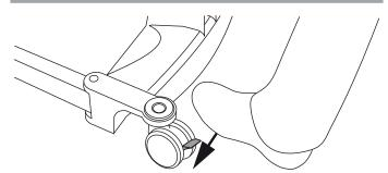
Rear wheels/castors are equipped with brakes. Step on lever to lock brakes. Flip up to unlock.
