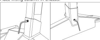
Lock the lift column in place by fastening the two hexagon socket screws in front and rear of the chassis.
