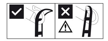
The suspensions hook design prevents sling to be inadvertently detached when mounted correct.
