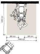
Grey area shows the minimum working area required for the staff to be able to use the mechanical aids in an ergonomic way from one side.
